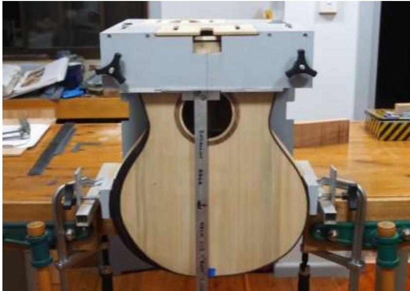
ROUTING THE BODY AND NECK JOINT
