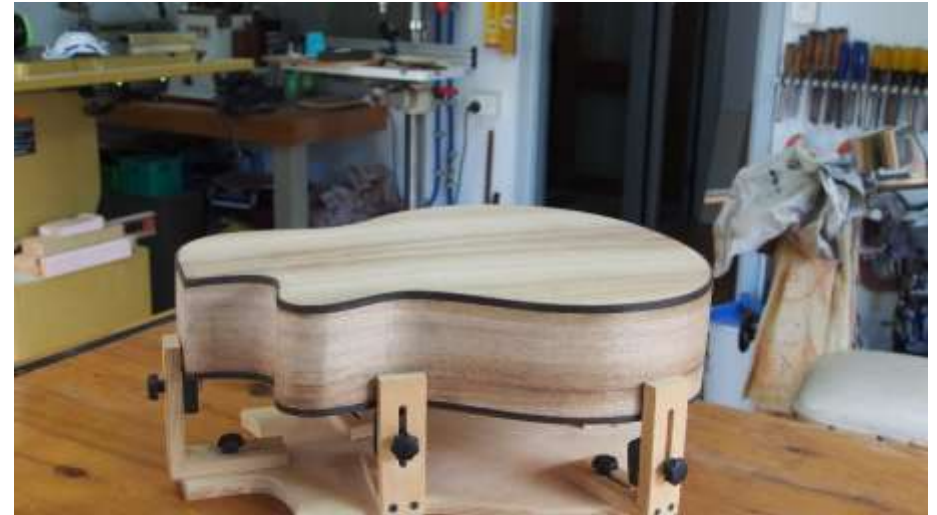
ALL BINDINGS FLUSHED AND CLEANED TO THEIR ADJOINING EDGE FACES
