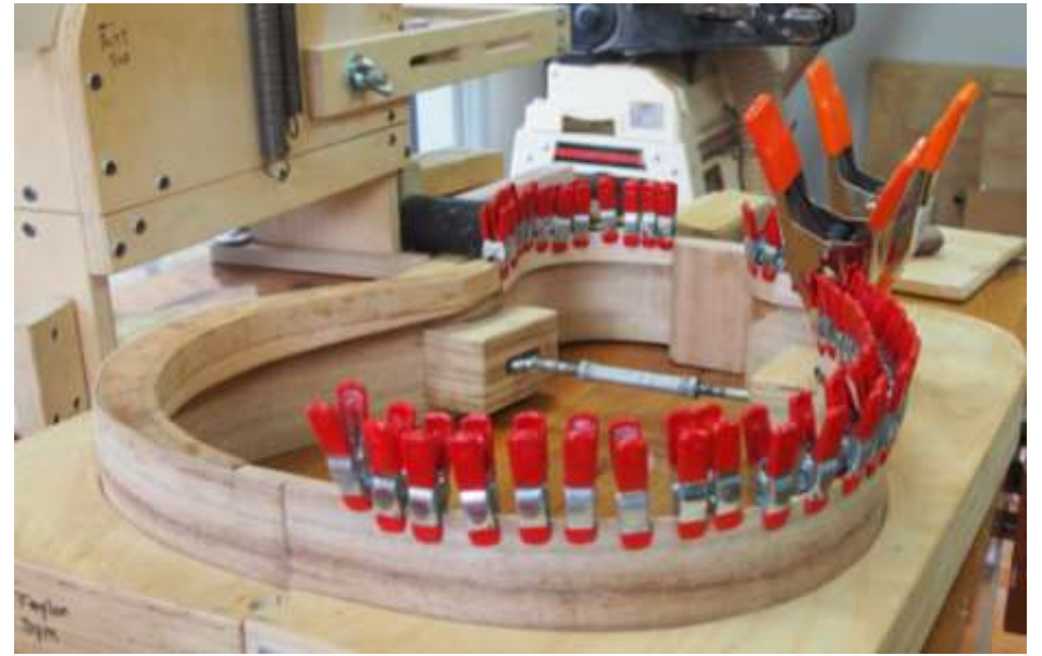
GLUEING THE SIDE LININGS AS LAMINATIONS
