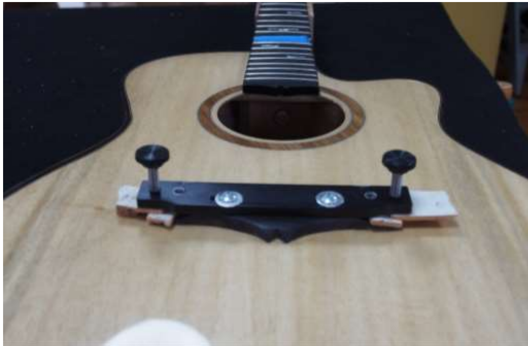
GLUEING THE BRIDGE TO THE GUITAR TOP
