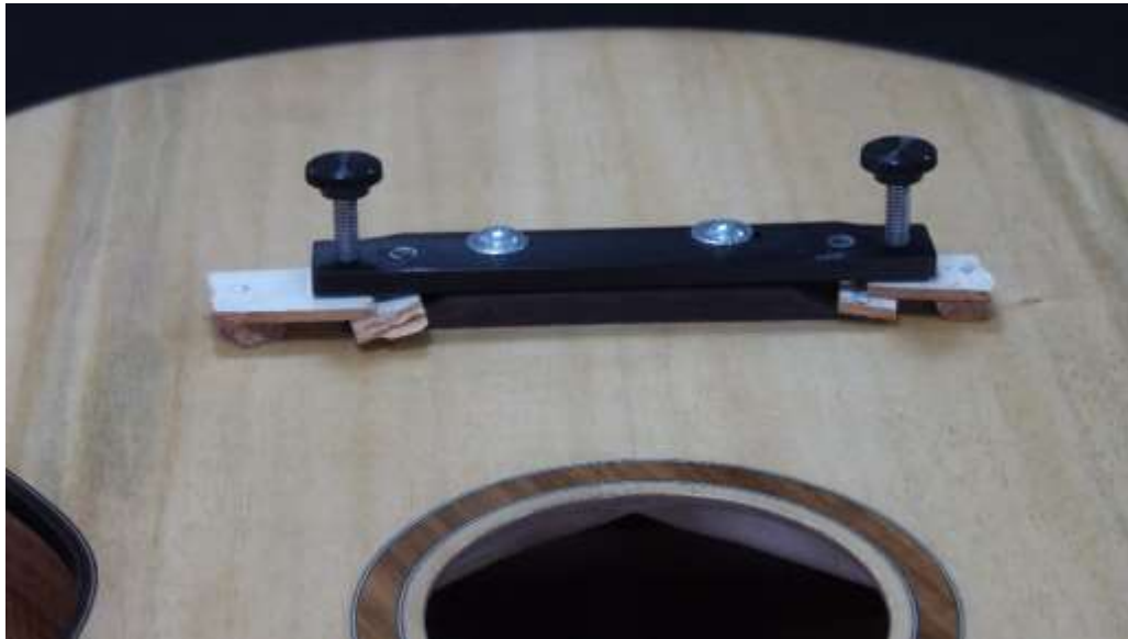
GLUEING THE BRIDGE TO THE GUITAR TOP
