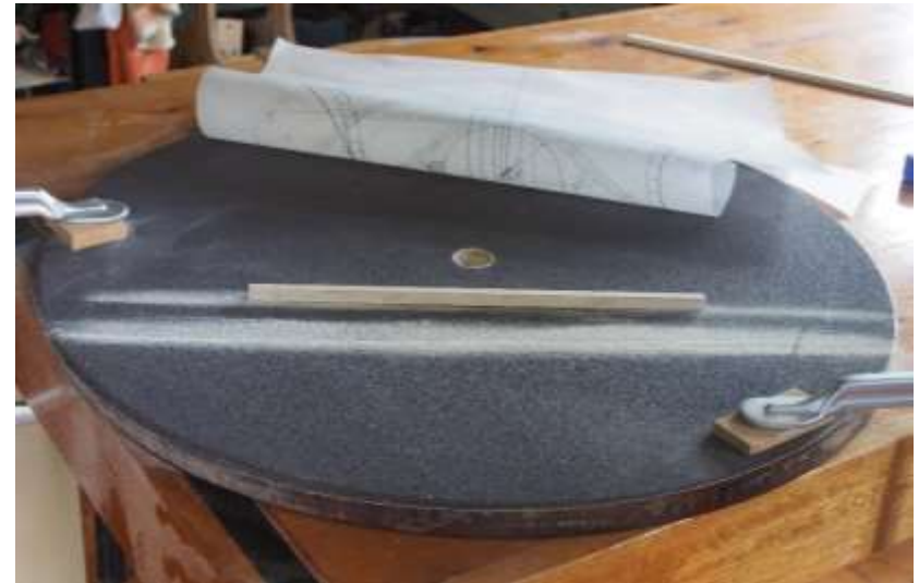
MAKING THE GUITAR BODY BRACING AND THEN RADIUS SANDING THE BRACES TO FIT THE 'TOP' & 'BACK'
