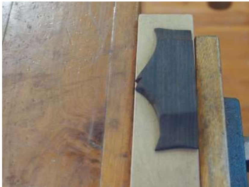
MAKING THE MACASSAR EBONY BRIDGE TO FIT THE 28FT CURVED TOP
