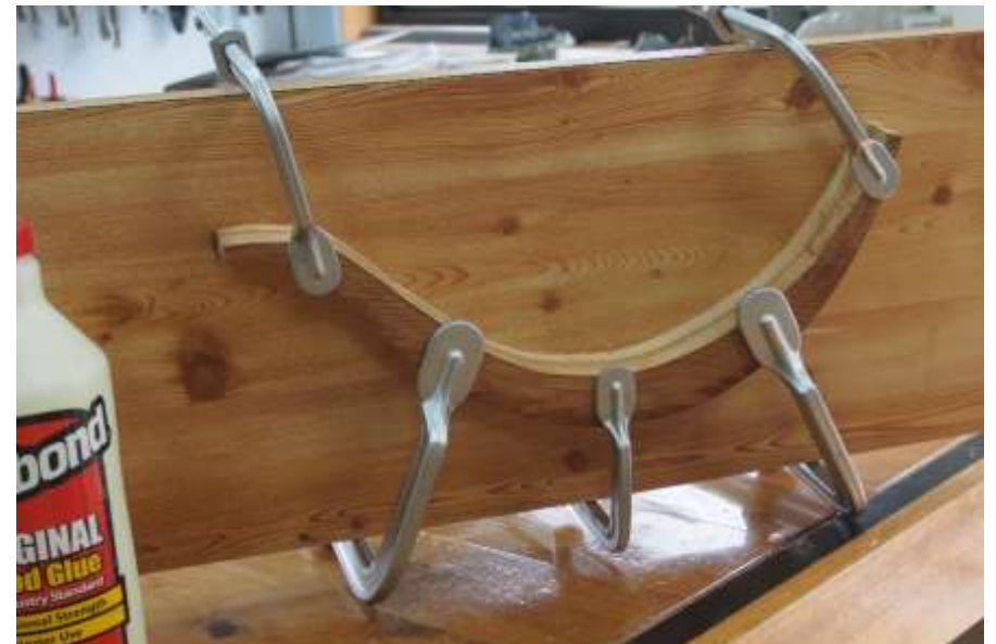
MAKING THE LINING FOR THE STREAMLINE ARM BEVEL REST
