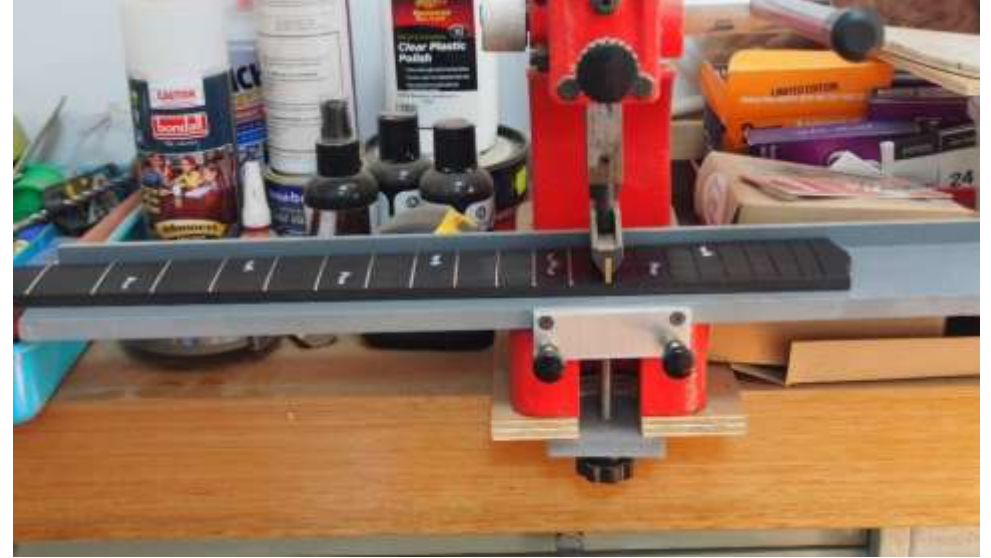
PRESSING THE FRETS TO THE FINGERBOARD
