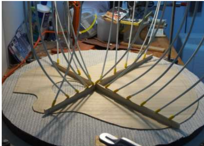
GLUEING THE 'TOP' BRACES WITH THE 28 FT RADIUS DISH IN THE 'GO BAR' CLAMPING JIG
