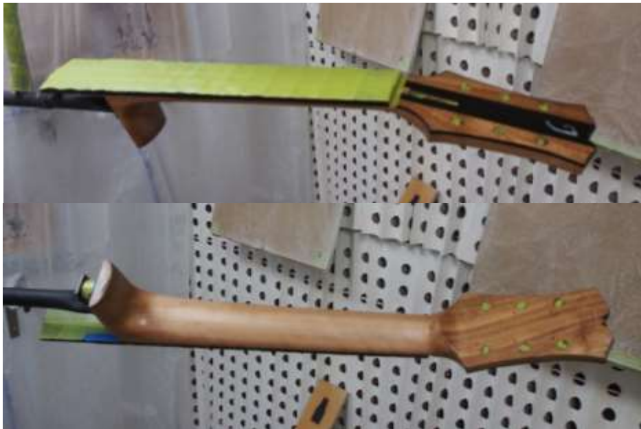
SPRAYING THE SEALER COAT
