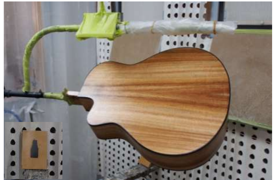
SPRAYING THE SEALER COAT
