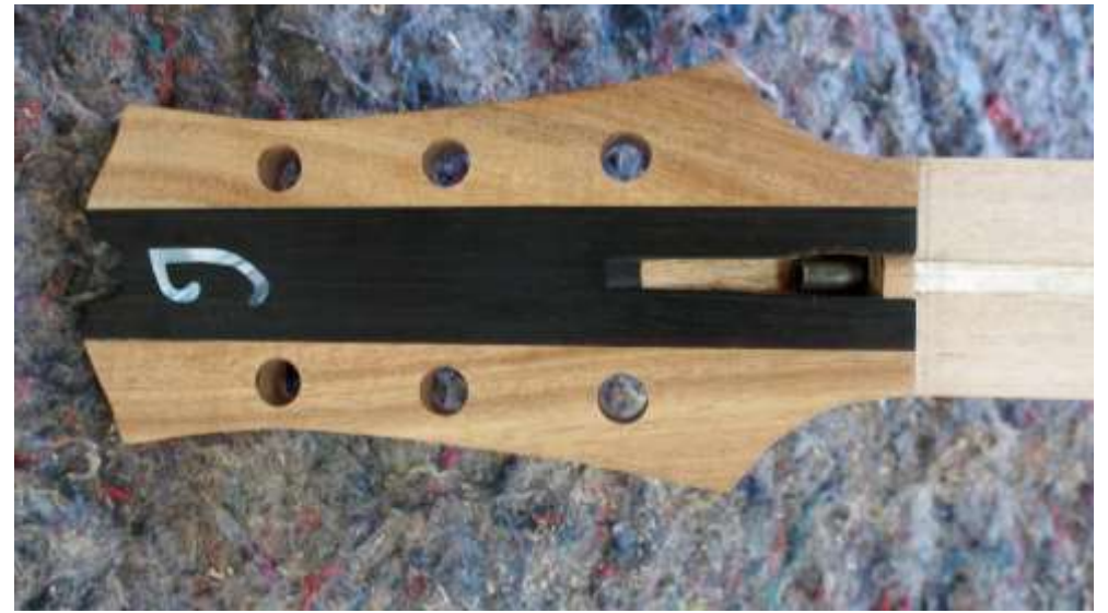
FITTING THE GOTOH 510 TUNERS
