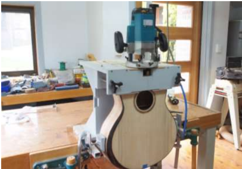
ROUTING THE BODY AND NECK JOINT
