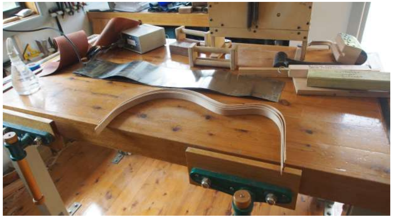
BENDING THE SIDE LININGS FOR LAMINATION PAGE 16
