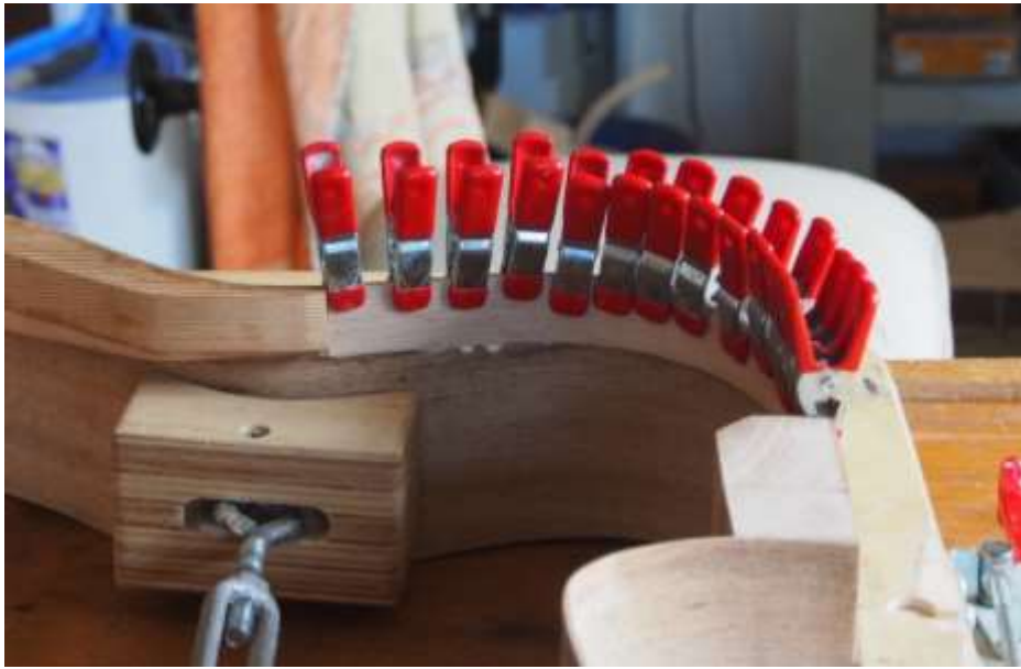
GLUEING THE SIDE LININGS AS LAMINATIONS
