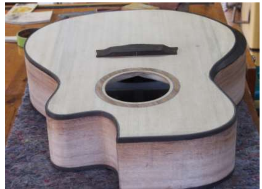
MAKING THE MACASSAR EBONY BRIDGE TO FIT THE 28FT CURVED TOP
