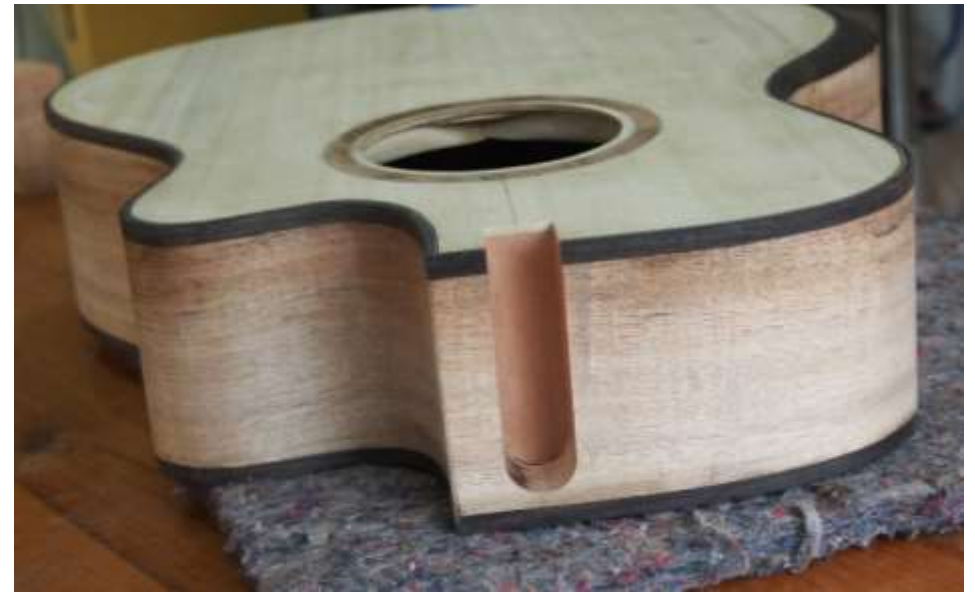
ROUTING THE BODY AND NECK JOINT
