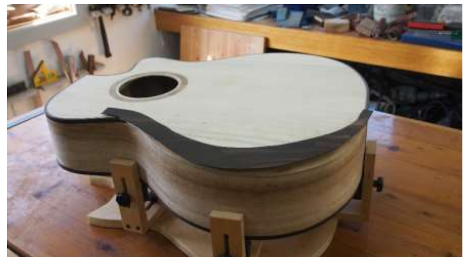
LOCATING THE CUTOUT MACASSAR EBONY VENEER ON THE ARM REST BEVEL
