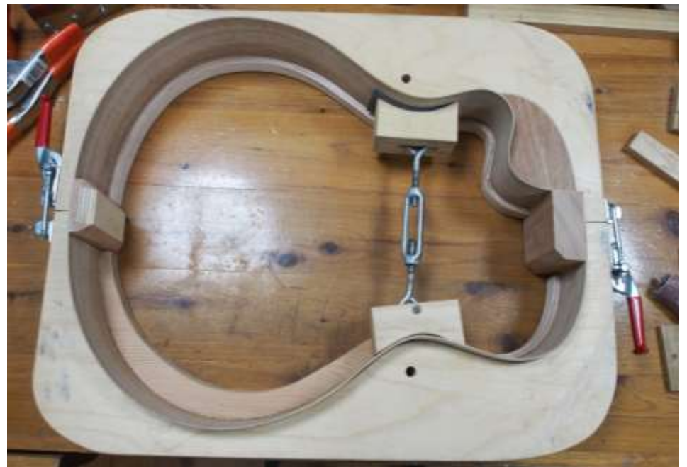
GLUEING THE SIDE LININGS AS LAMINATIONS
