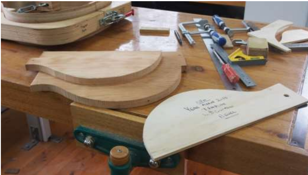
MAKING THE LINING FOR THE STREAMLINE ARM BEVEL REST
