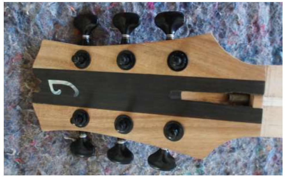
FITTING THE GOTOH 510 TUNERS
