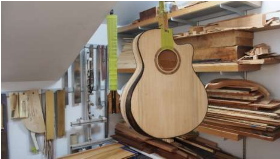
MASKING THE NECK & BODY READING FOR SPRAYING
