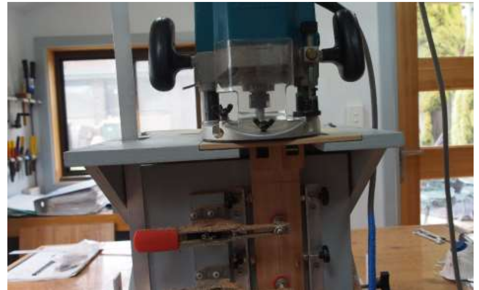
ROUTING THE BODY AND NECK JOINT
