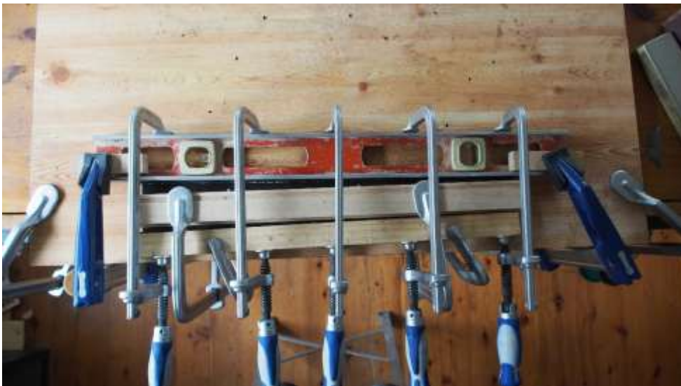
GLUEING THE FINGERBOARD BINDINGS
