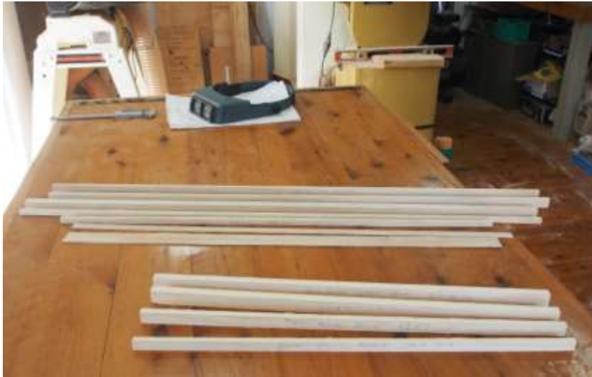
MAKING THE GUITAR BODY BRACING AND THEN RADIUS SANDING THE BRACES TO FIT THE 'TOP' & 'BACK'
