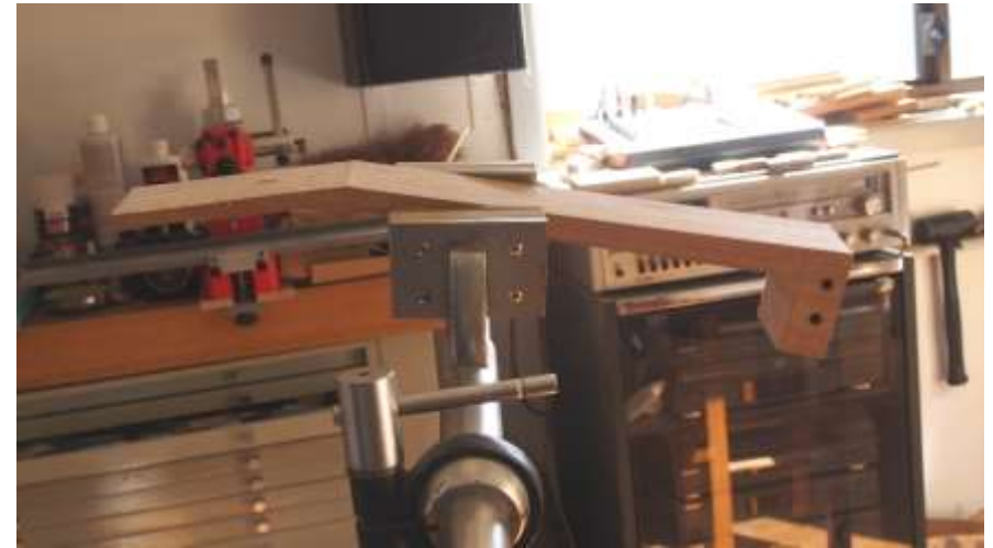
PREPARING THE NECK FOR THE BOLT ON FITTINGS
