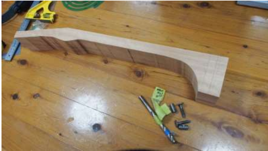
PREPARING THE NECK FOR THE BOLT ON FITTINGS
