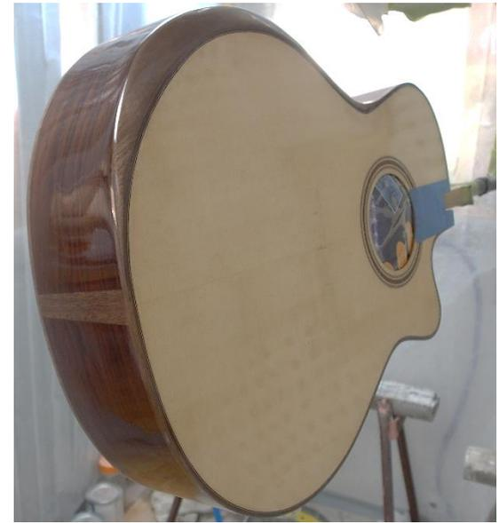
**SPRAYED 2 SEALER COATS & FIVE WET NITRO LACQUER COATS UNDERTAKEN. FINAL SIXTH THIN COAT TO BE ADDED**
