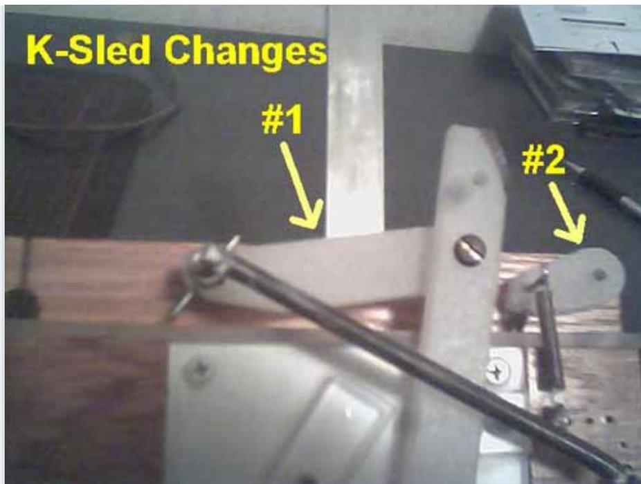
Now all that you need to do is fit some kind of hooks to hold the rubber bands or spring in place, fit the "Stop" block, and the "Strip Guide Holder" align the jig back onto your bandsaws table checking all is in order and finally fit the mitre bar to the Sub-base , change out the small 20mm particle board screws that were holding the 4" x 4" Lexan plate to the Indexing Base so that all is secure, dimension down some stock and cut some kerfing.
