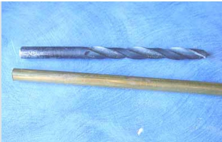
Once you have drilled your Lexan (clamped securely and in safe increments) out to 9/32" you simply use your bandsaw with that fine tooth metal blade, to cut a small piece of the brass tubing just a tiny bit shorter than the lexan is thick. Gently clean off the burr from your little brass bushing with a fine needle file (not too much now, we want a press fit), and press it home into the hole you drilled in the Lexan. This piece is now ready to accept a 1/4" bolt or threaded rod as a shaft.
